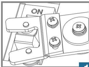
1 The design of the MCCB toggle operation mechanism allows for correct and smooth position switching in the on, off & trip status.
