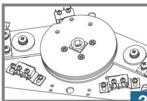
3 Aided by micro switch position detection, the ATS switching position operates to the accuracy required.
