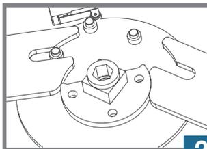
2 The optimised cam transmission mechanism design ensures the reliability of the mechanical interlock and at the same time helps to extend the mechanical life to over 10,000 operations.
