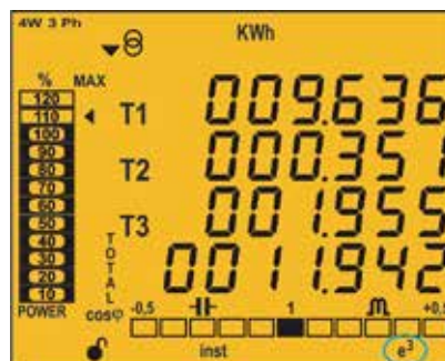
Figure 30: CVM-C10 screen with the e 3 profile.
